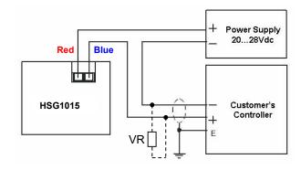
VR - for achieving a DC voltage signal, as alternative to the standard 4...20mA signal, connect a fixed resistance across the 'customer' input:
